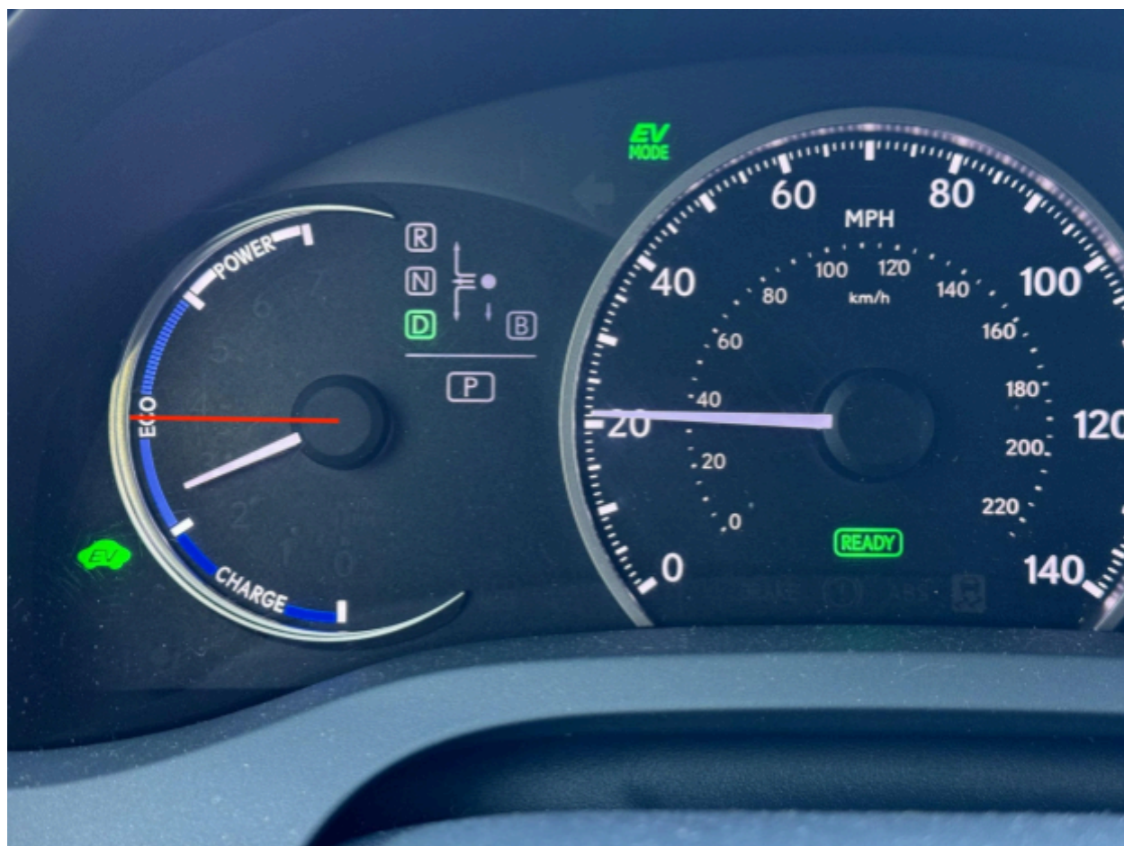
The line (in red) on the tachometer that cannot be crossed to keep the vehicle in EV Mode.
